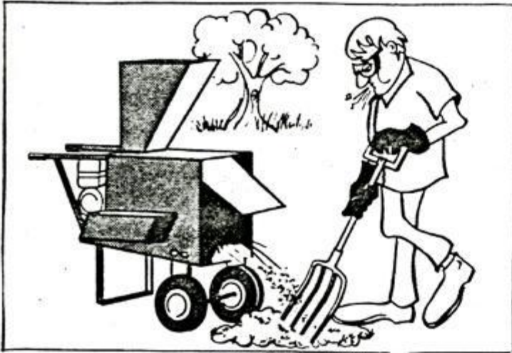
Do clear discharge area of machine with spade, rake or long handle tool.
