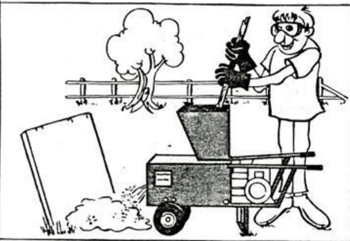
Use stick, never hands, if material bridges in hopper. Do keep people away and discharge shredded material into compost heap or fixed known obstruction.
